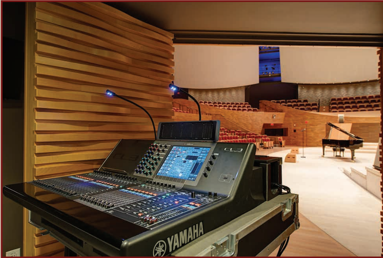
The Yamaha CL-3 production console for stage-monitor mixing.
