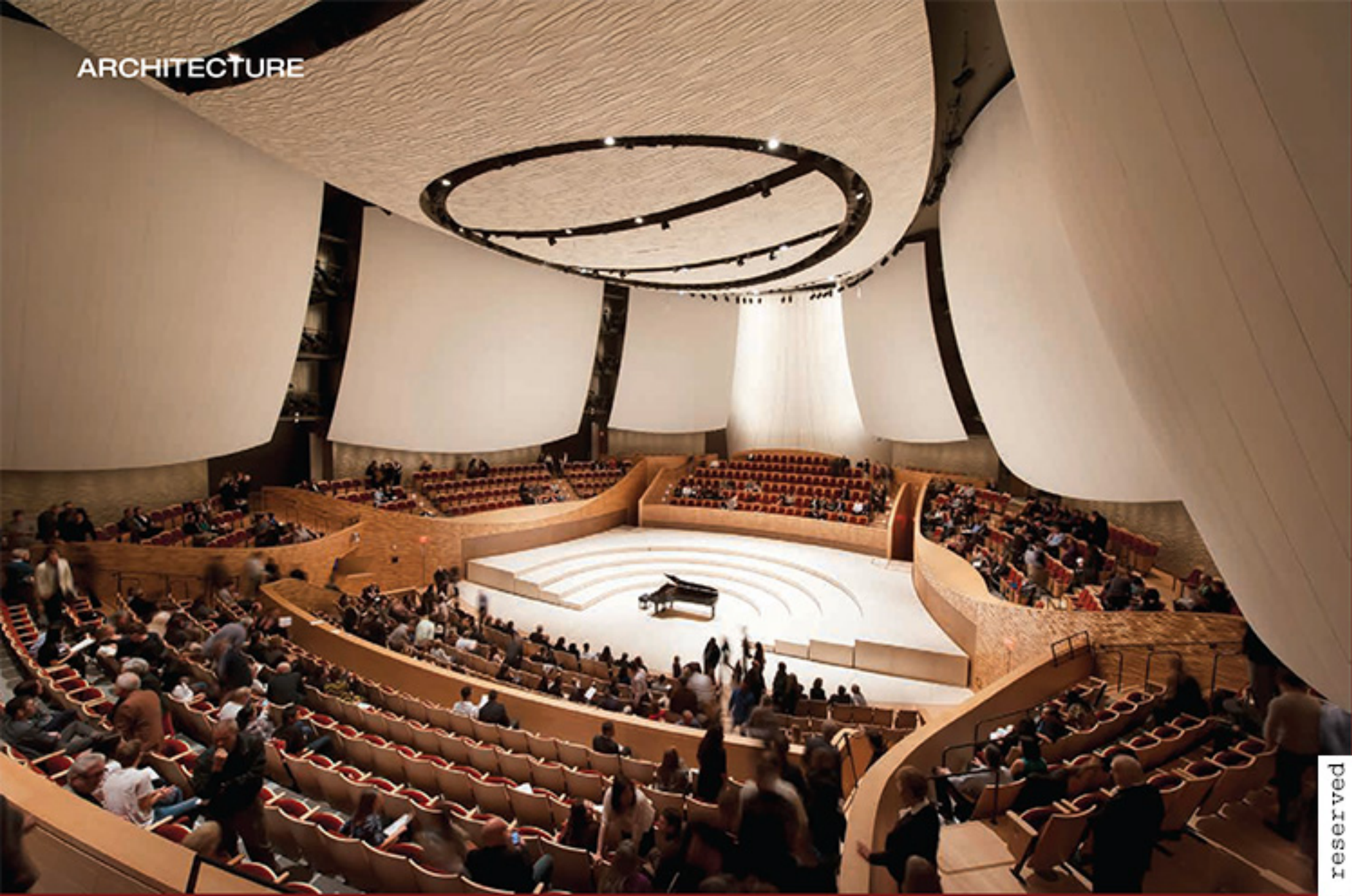
Low walls embracing each seating section are angled and articulated with beech wood, which has a specific density and textured surface strategically designed to reflect and disperse sound.
